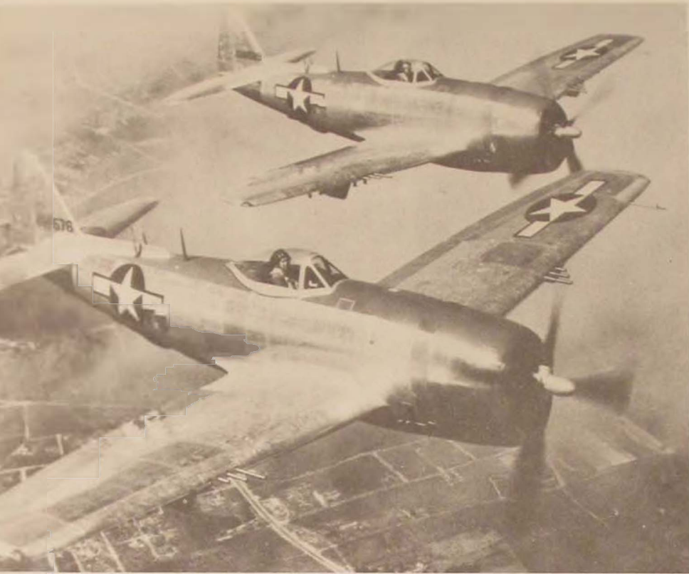
P-47 Thunderbolts (left), with their eight machine guns and rugged construction, were well suited for strafing and bombing missions. . . . The lighter and faster P-51 Mustangs (below) were more vulnerable to ground fire but better at aerial combat.
